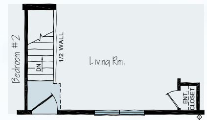
OPT. BASEMENT STAIRWAY LAYOUT
